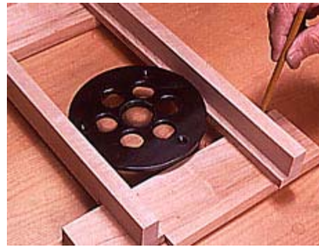
1--Make the carriage tracks and place them on the track joiners. Adjust spacing and then mark for joiner dadoes.
