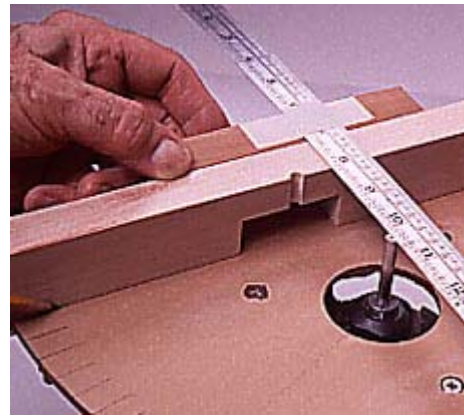
2--Install a 1/4-in. rod in router and attach router and fence to the new base. Seat rod in half hole to find zero mark.
