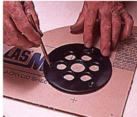
1--Remove the base from the router and use it to mark the screwholes and the router-bit hole on the acrylic sheet.
