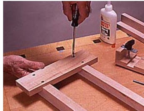
2--After the dadoes have been cut in the joiners, secure one joiner with glue and screws. Opposite joiner is adjustable.
